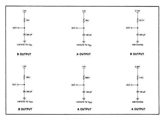
Figure 5. Test Load Circuits
